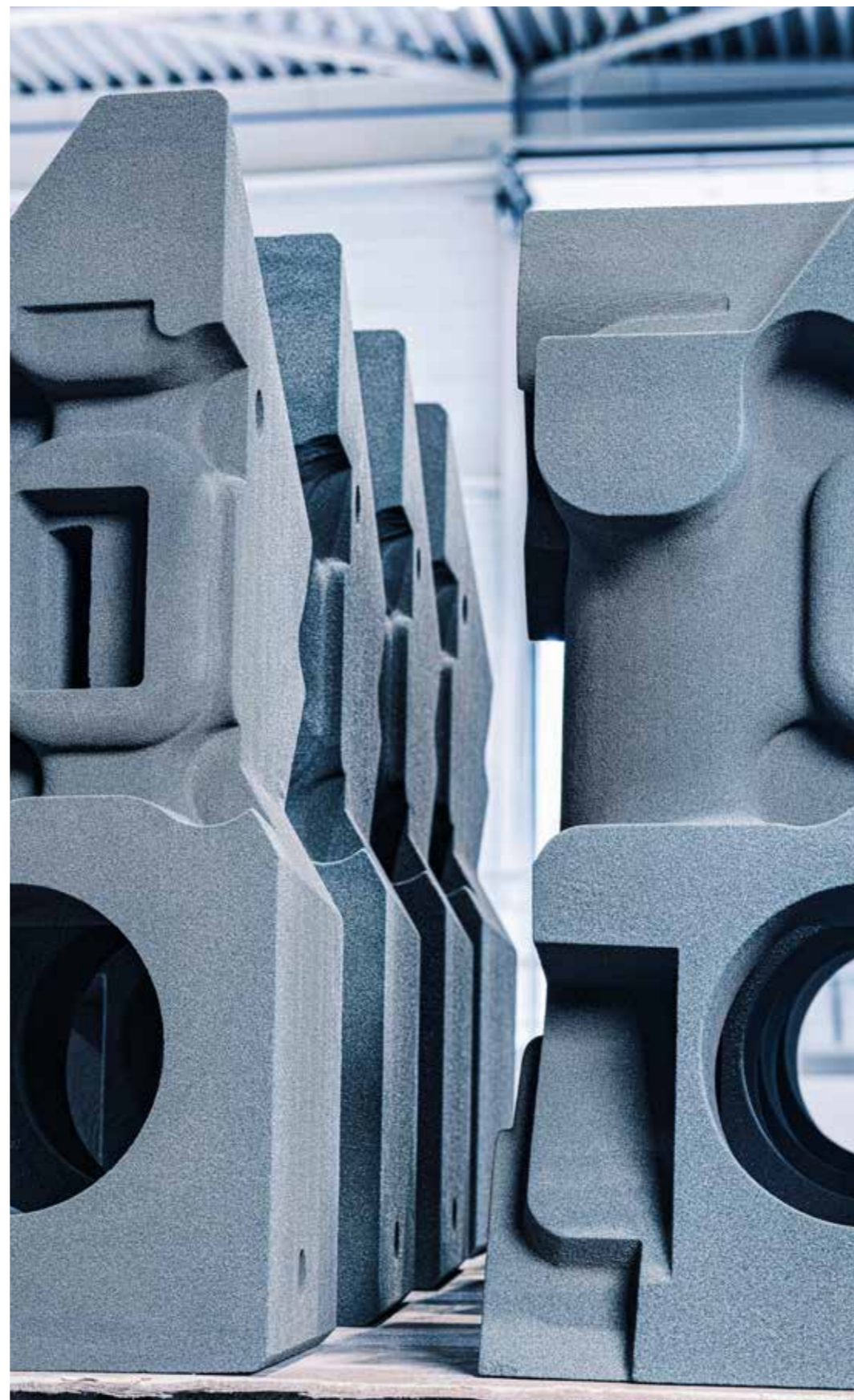
High-precision 3D-printed sand cores for use in the railway industry
