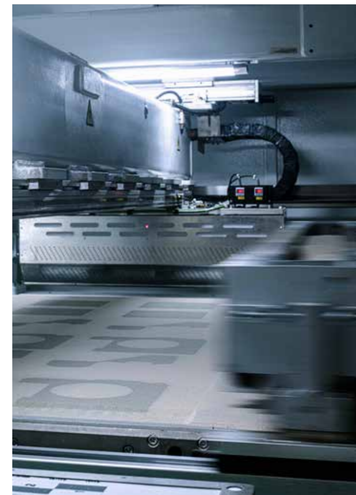
3D sand printing process
